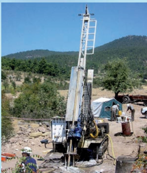
Diamond drilling rig at the Arzu South Vein.
